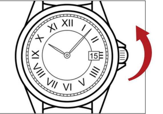
It operates without batteries and winds automatically. But correct manual winding is essential, which can effectively reduce time deviation.
